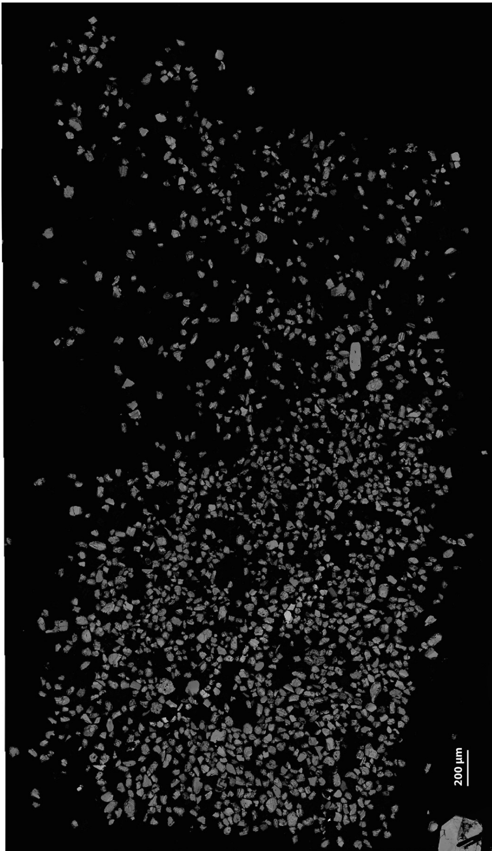
Figure 17F: Unlabeled BSE images of zircon grain mount for sample KRCD
