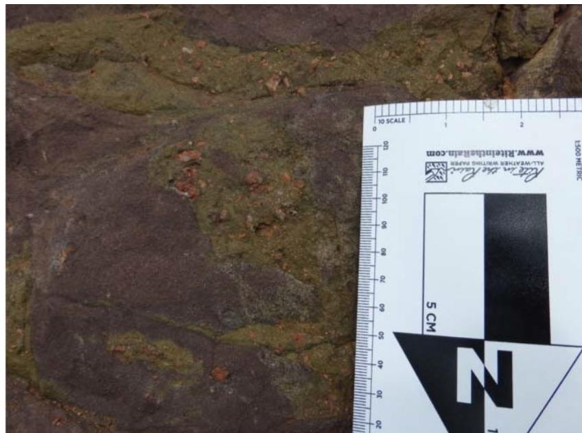
Figure 16: This photo shows the second type of parent body observed at Pine, CO. Green, irregular mass of material that is mixed within parent sandstone body. The green color corresponds to chemically altered material that has a swirled, irregular contact with the Tava quartz sandstone. Analysis using the XRF shows the green material to be chlorite.
