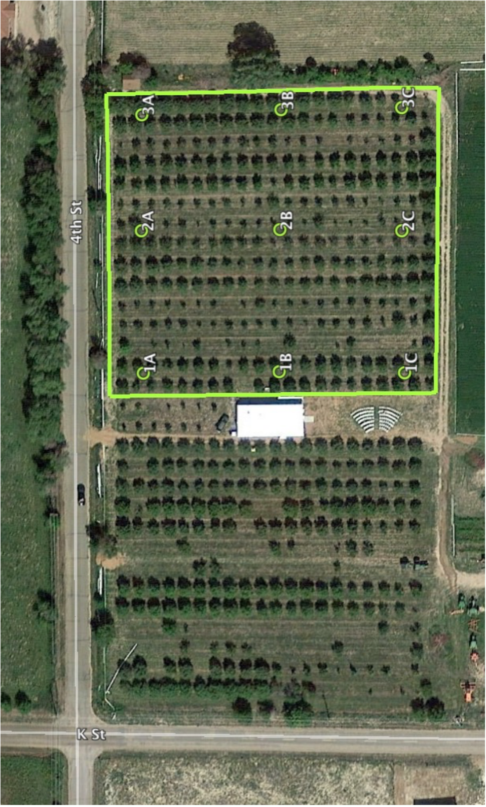
Figure 18) Locations of Grid Sonic Anemometer Placement
