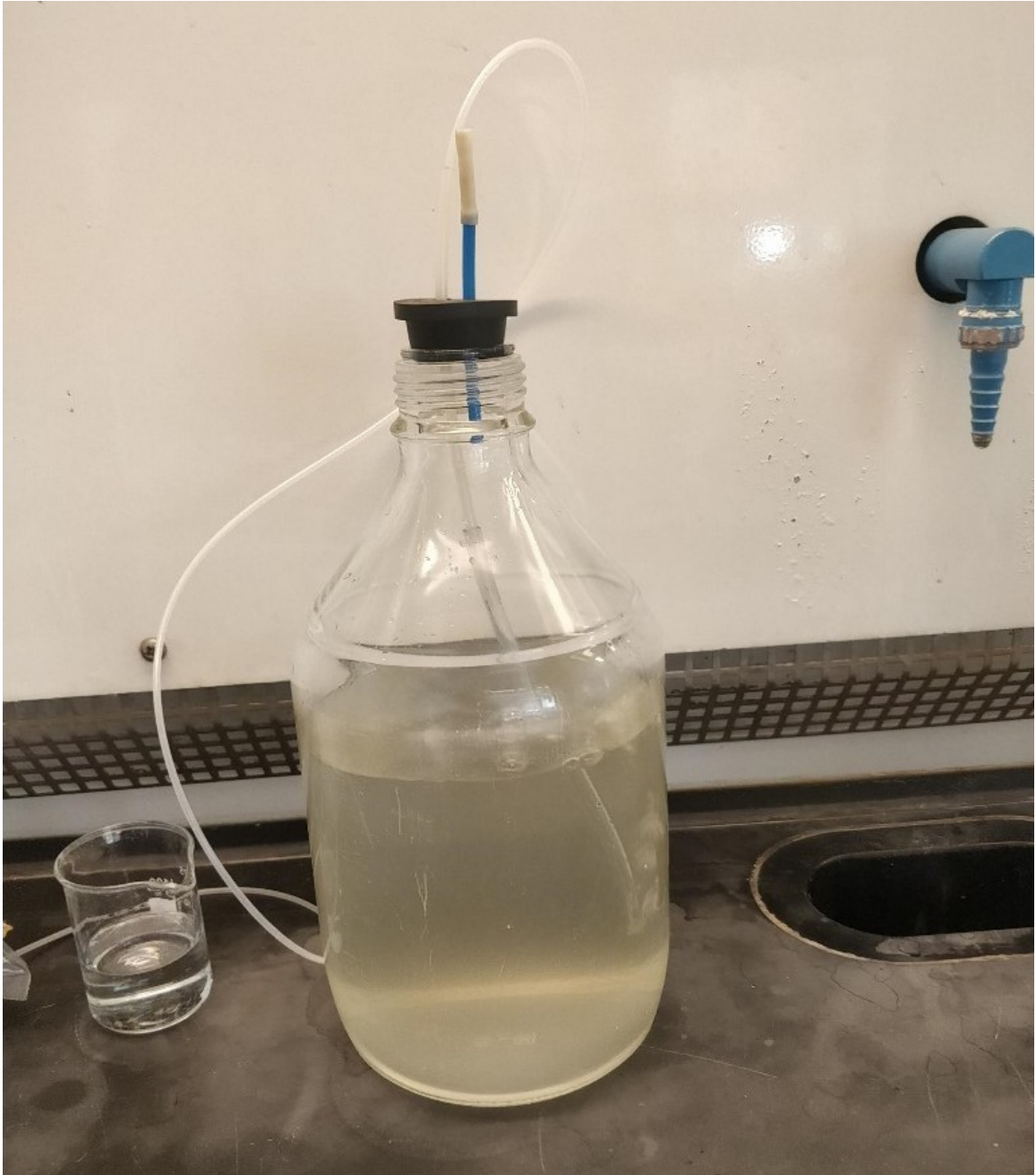
Figure 1: Sample 1, TIE level 1 Aeration setup
