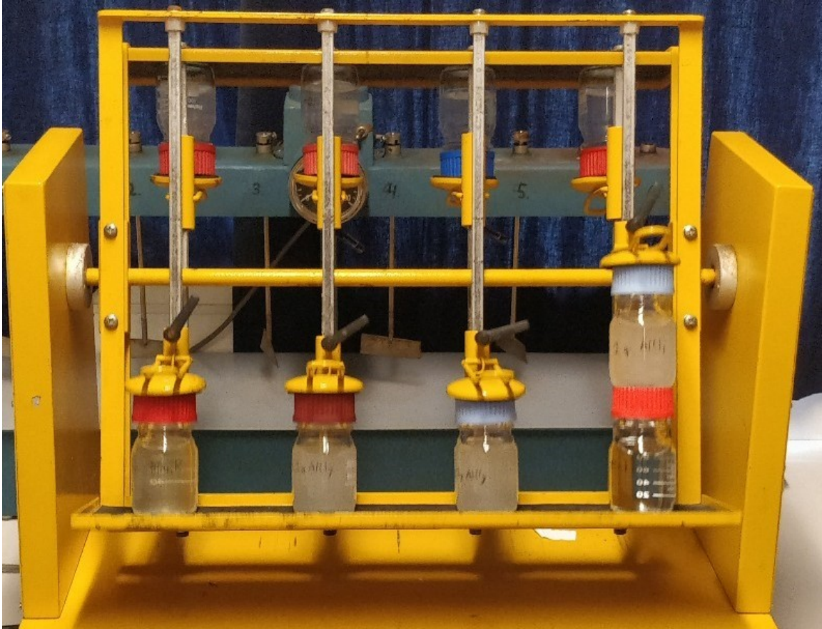
Figure 2: 24 hr. End-over-end shaker for TIE treatments
