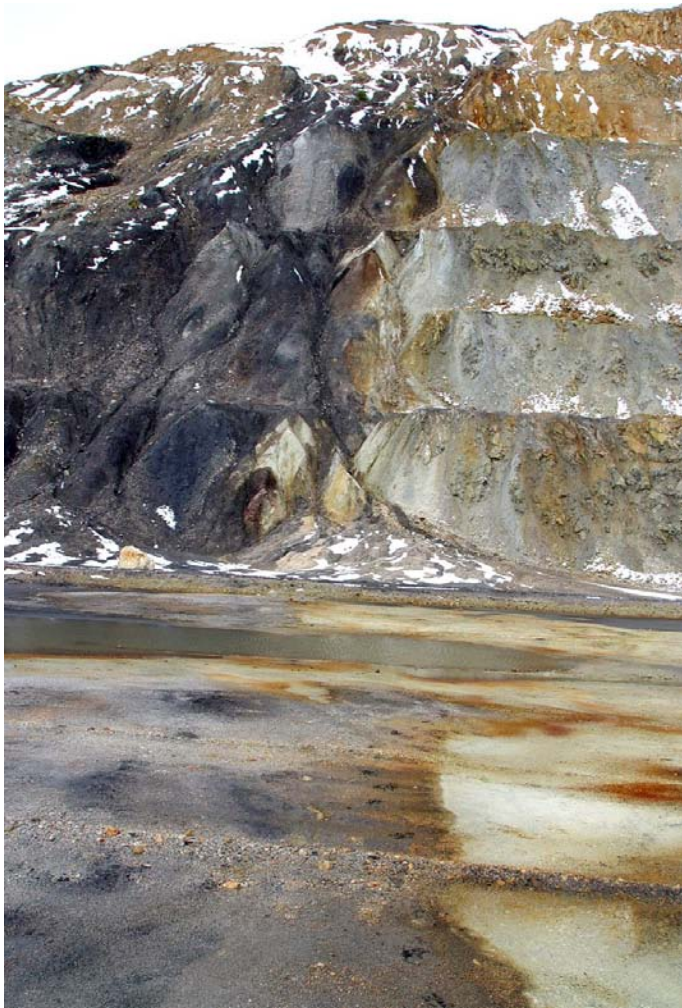
Figure 4. The Mosquito fault in the north wall of the Climax Pit, juxtaposes Minturn Formation (left) against lighter Precambrian granite and Tertiary porphyry (right). Here the fault zone dips steeply west and is approximately 50 ft wide. Widmann and others (2004a) describe the eastern margin of the fault zone as a 1 to 1.5 foot wide zone of light-gray to white, clayey fault gouge, probably derived from crushing and pulverizing of the Precambrian granite in the footwall block. The footwall block has been altered to a jasperoid mass for a distance of at least 50 ft from the fault. The wide fault zone is mainly composed of 3-6 foot wide slivers of Minturn Formation. The slivers are lens shaped, elongated parallel to the fault zone, and appear to have tapered ends that dovetail into each other. Photo by Vince Matthews.
