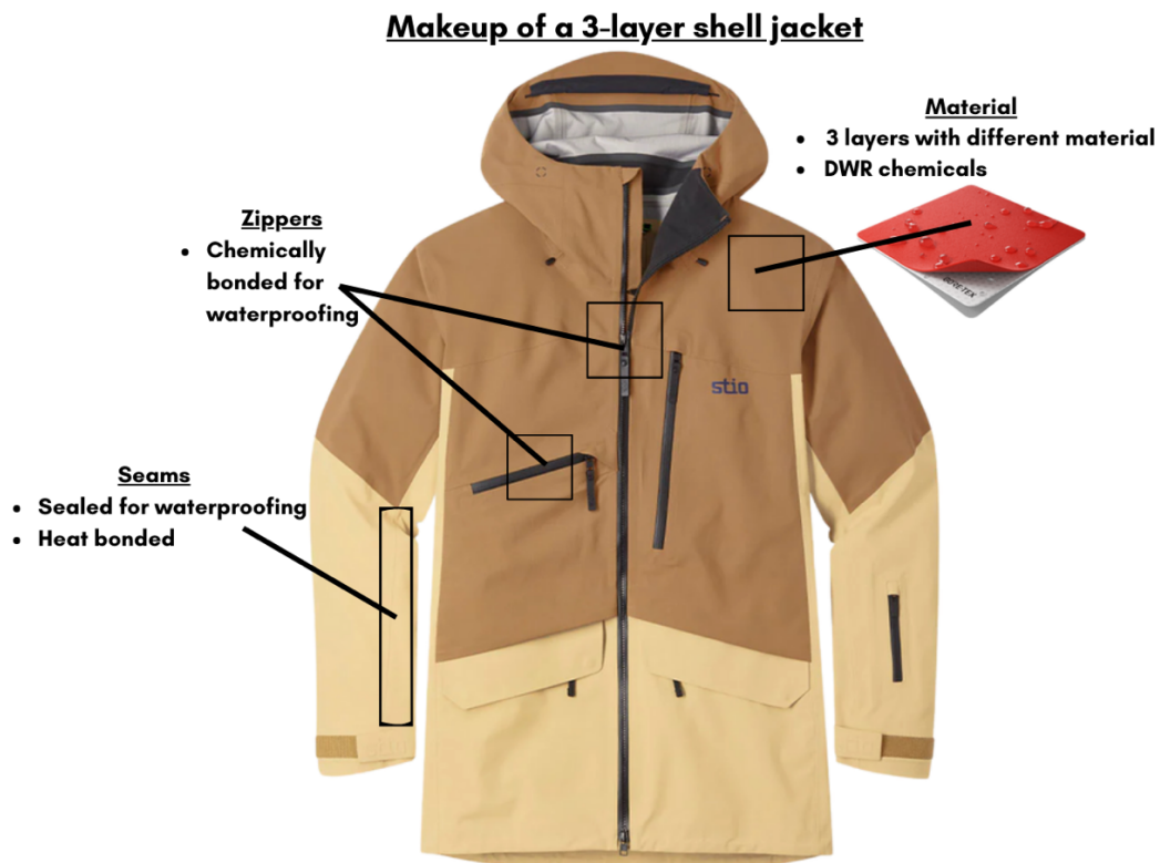
Figure 1. The components of a 3-layer shell jacket that challenges circularity
